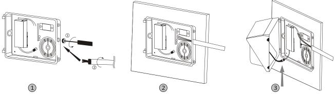
Step1. Loosen screws and remove the front lens set carefully from the back plate.
