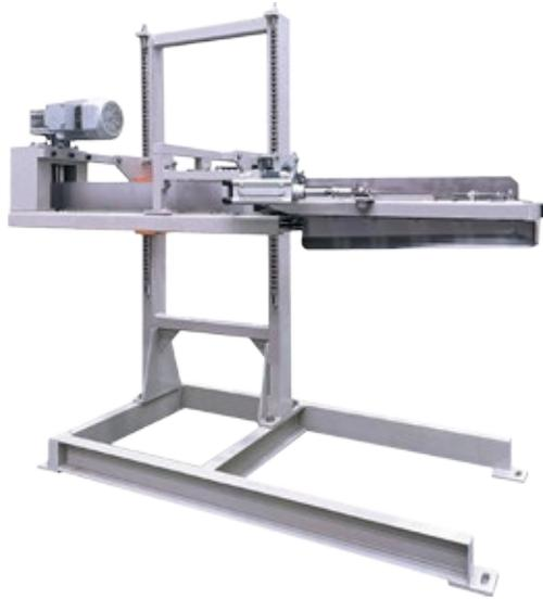
This model is a special model for automatic bag clamping and bag feeding. It is suitable for working with multi-station weighing scales. The front-end bag-clamping mechanism transmits the packaging bag to the bag-feeding mechanism through photoelectric induction, and sends it to the back-end sealing equipment to complete the packaging bag sealing. Work.
