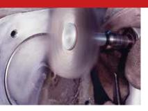
Stem-mounted Nylon Brushes are used on a variety of portable tools and drills. These radial nylon abrasive wire brushes are available in 80grit 120grit 150grit 180grit and 240 grit, bristle diameter is from 0.7mm - 1.8mm.
