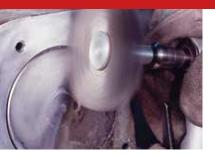
crimped wire wheels are used on a variety of portable tools and stationary machines. These radial brushes are available in heat-treated Steel, Type 304 Stainless Steel .
