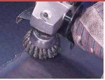
HOYIN's wire cup brushes are intended primarily for use on portable power tools for addressing larger surface areas more efficiently than a wheel brush. Cup brushes are designed for smooth, efficient operation on angle grinders to make quick work of large jobs.
