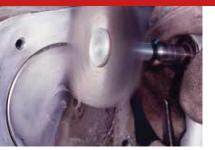
crimped wire wheels are used on a variety of portable tools and stationary machines. These radial brushes are available in heat-treated Steel, Type 304 Stainless Steel and Coarted Brass.
