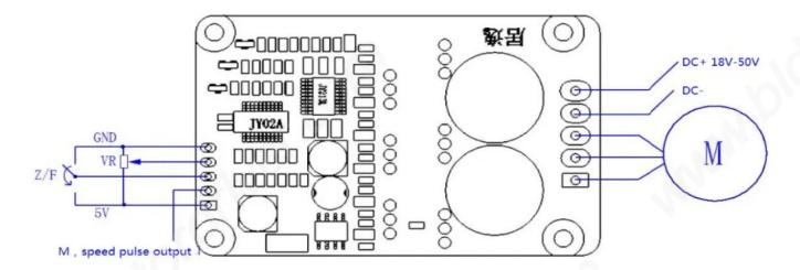
5V -----Driver board internal output voltage
