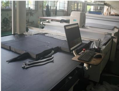
Automatic cutting machine which can cut more than 100 layers in one time
