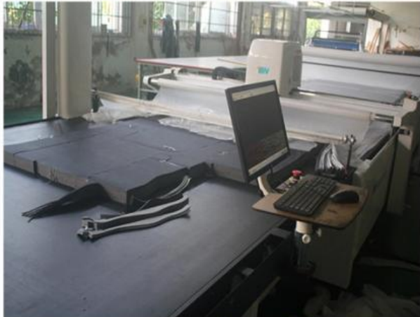
Automatic cutting machine which can cut more than 100 layers in one time
