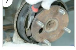
Remove the brake shoe with the slotted screwdriver.
