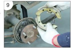
12. Install the shoe retainer with the long flat nose pliers.
