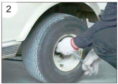
5. Raise the frame of the rear suspension with the jack to hang the rear wheel in the air.
