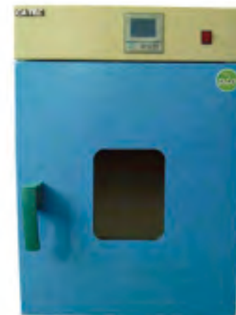
VERTICAL BLAST DRYING OVEN(250 °C
